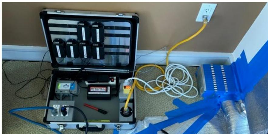
**Figure 5.** A temperature sensor control unit.
