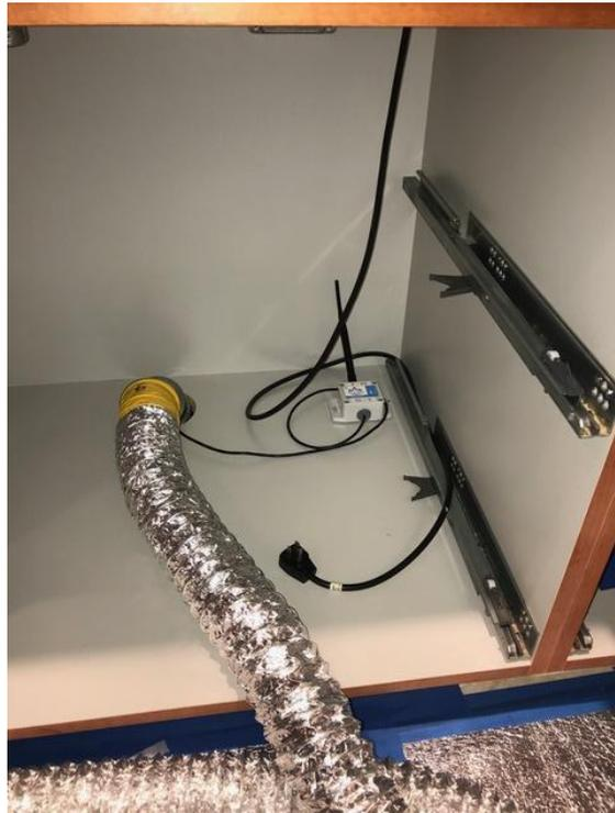
**Figure 3.** In each improved treatment home, probes (right) were placed in toe-kick voids for temperature monitoring and recording. Flexible duct pipes (left; with yellow cloth) were placed in toe-kick voids to direct heated air.
